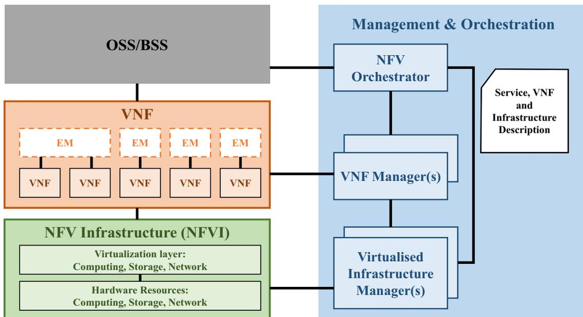
**Fig. 3** High-level overview of NFV architecture (reconstructed from [12, 14, 15])
