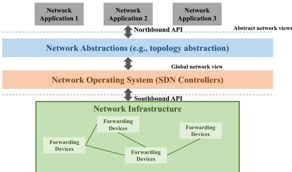
Fig. 2 High-level overview of SDN architecture (reconstructed from [13])
